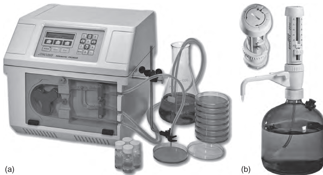
Fig. 4.6. Automatic Dispensers. (a) The Perimatic Premier, suitable for repetitive dispensing and dilution in the 1- to 1000-mL range. If the device is used for sterile operations, only the delivery tube needs to be autoclaved. (b) Zippette bottle-top dispenser, suitable for the 1- to 30-mL range; autoclavable. (Courtesy of VWR-Jencons.)
