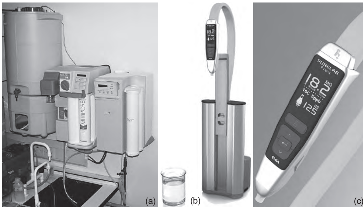
Fig. 4.15. Water Purifier. (a) High output. Tap water first passes through a reverse-osmosis unit on the right and then goes to the storage tank on the left. It then passes through carbon filtration and deionization (center unit) before being collected via a micropore filter (Millipore Milli-Q). Current models have integrated conductivity and TOC monitoring (Courtesy of Beatson Institute.) (b) Smaller self-contained bench-top unit (Elga Pureflex). (c) Handset with readout of resistivity and TOC. (b, c, courtesy of Elga.)
