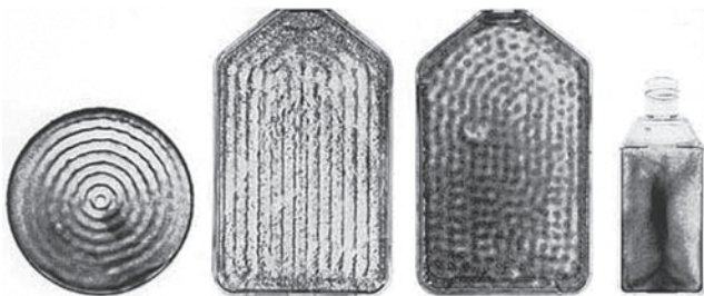
Fig. 7.10. Nonrandom Growth. Examples of ridges seen in cultured monolayers in dishes and flasks, probably due to resonance in the incubator from fan motors or to opening and closing of the incubator doors. (Courtesy of Nunc.)
