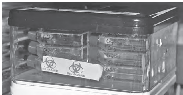
Fig. 5.11. Boxed Dishes. A transparent box, such as a sandwich box or cake box, helps protect unsealed dishes and plates, and flasks with slackened caps, from contamination in a humid incubator. This type of container should also be used for materials that may be biohazardous, to help contain spillage in the event of an accident. (Material known to be biohazardous would need a sealed container and a separate incubator.)
