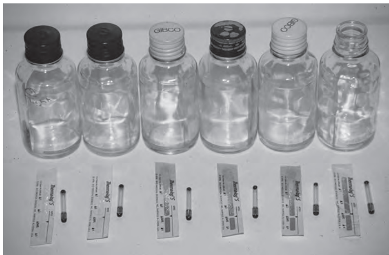
Fig. 10.3. Sterilizing Capped Bottles. These bottles were autoclaved with Thermalog sterility indicators inside. Thermalog turns blue with high temperature and steam, and the blue area moves along the strip with time at the required sterilization conditions. The cap on the leftmost bottle was tight, and each succeeding cap was gradually slacker, until finally no cap was used on the bottle farthest to the right. The farthest left bottle is not sterile because no steam entered it. The second bottle is not sterile either, because the liner drew back onto the neck and sealed it. The next three bottles are all sterile, but the brown stain on the indicator shows that there was fluid in them at the end of the cycle. Only the bottle at the far right is sterile and dry. The glass indicators (Browne's tubes) all implied that their respective bottles were sterile. (See also Plate 22a.)
