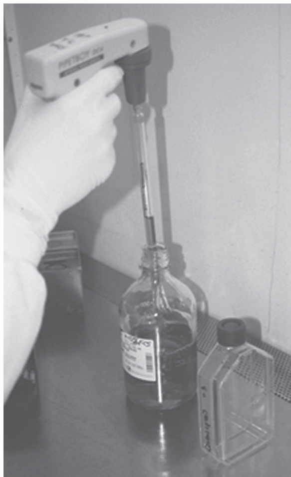
Fig. 4.2. Pipette Controller. Motorized pipetting device for use with conventional graduated pipettes.
