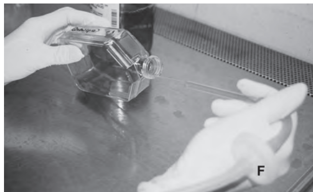
Fig. 5.12. Gassing a Flask. A pipette is inserted into the supply line from the CO 2 source, and 5% CO 2 is used to flush the air out of the flask without bubbling through the medium. The letter “F” indicates a micropore filter inserted in the CO 2 line.
