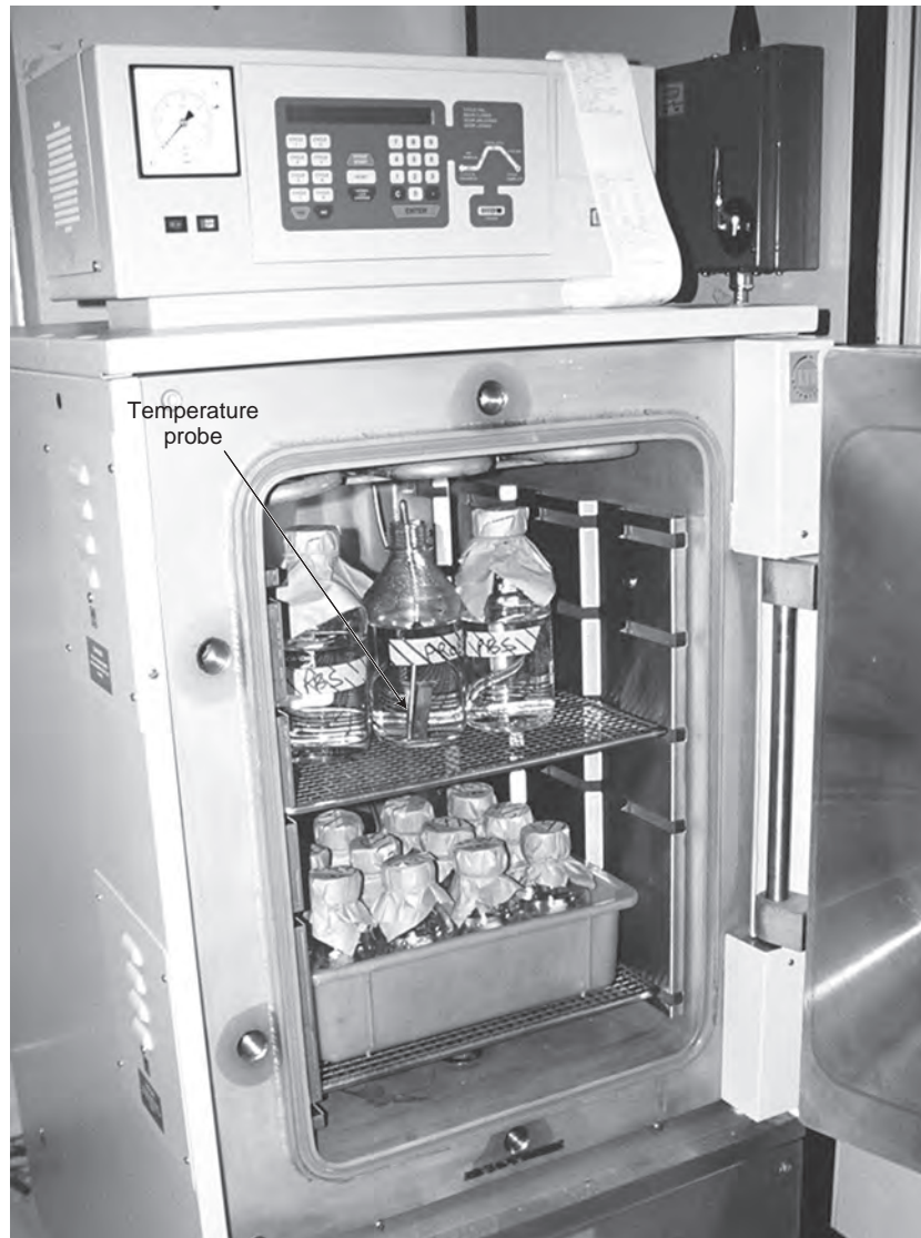
Fig. 4.17. Freestanding Autoclave. Medium-sized (300 L; 10 ft 3 ) laboratory autoclave with square chamber for maximum load. The recorder on the top console is connected to a probe in the bottle in the center of the load. (Courtesy of Beatson Institute.)
