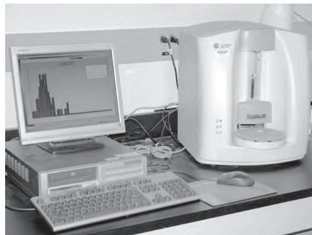
Fig. 20.5. Beckman Coulter Vi-CELL. An undiluted cell suspension is placed in a cup in the sample holder, sampled by the counter (right), mixed with Trypan Blue, and analyzed in a flow cell. The output appears on the display (left) as a graphic of cell size distribution or a microscope view of the cells with live cells circled in green and dead cells circled in red. (Courtesy of ATCC.)
