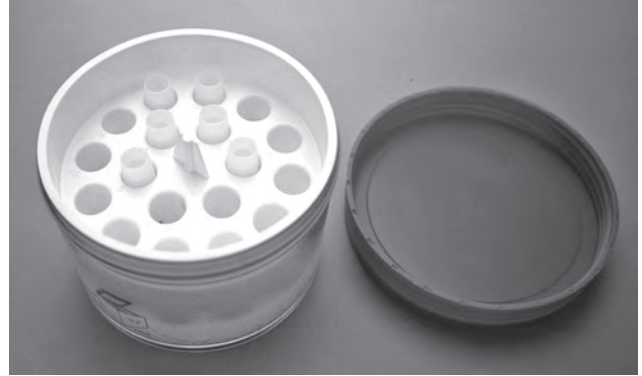
Fig. 19.4. Nunc Cooler. Plastic holder with fluid-filled base. The specific heat of the coolant in the base insulates the container and gives a cooling rate of about 1^{\circ}\text{C}/\text{min} in the ampoules.
