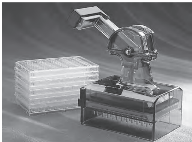
Fig. 4.8. Transfer Device. Transtar (Corning) for seeding, transferring medium, replica plating, and other similar manipulations with microtiteration plates, enabling simultaneous handling of all 96 wells. (Reproduced by permission of Corning Life Sciences.)
