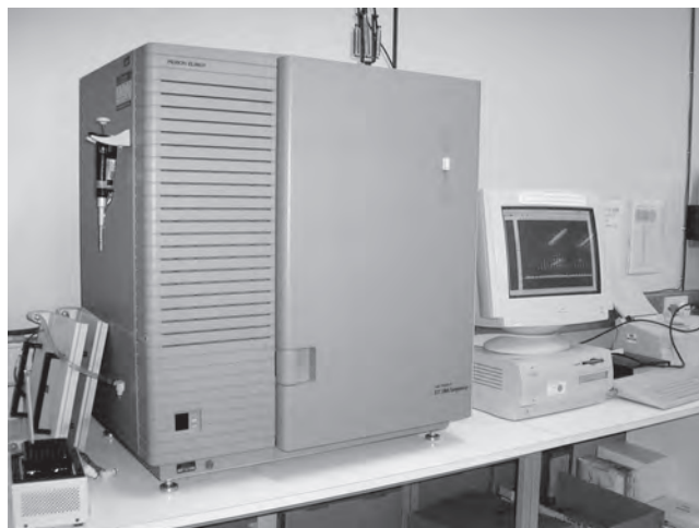
Fig. 15.10. DNA Sequencer. ABI 377 DNA sequencer using automated electrophoretic analysis on polyacrylamide gel to separate and quantify amplified STR sequences. (Photo courtesy of A. Meredith, LGC Promochem.)
