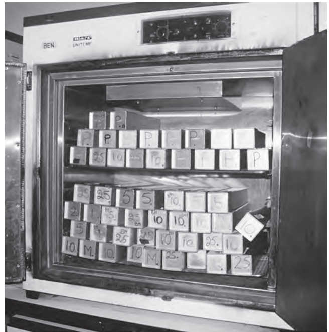
Fig. 10.7. Sterilizing Oven. Pipette cans are stacked with spaces between to allow circulation of hot air. Brown staining on front of oven shows evidence of volatile material from sterile-indicating tape, a problem when using tape in a hot oven.
