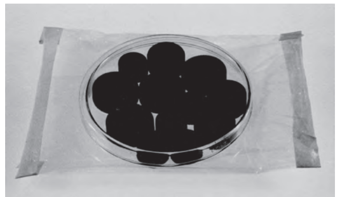
Fig. 10.8. Packaging Screw Caps for Sterilization. The caps are enclosed in a glass Petri dish, which is then sealed in an autoclavable nylon bag.
