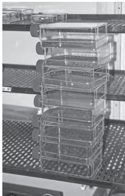
Fig. 5.10. Tilting Flasks. The air space inside a flask expands in the incubator or warm room. In large flasks, this causes the flask to bulge and will tilt the flasks, increasing the tilt with the height of the stack.
