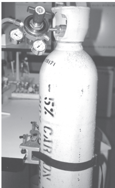
Fig. 6.3. Cylinder Clamp. Clamps onto edge of bench or rigid shelf and secures gas cylinder with fabric strap. Fits different sizes of cylinder and can be moved from one position to another if necessary; clamp is available from most laboratory suppliers.
