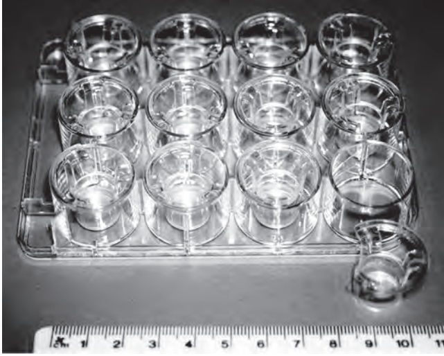
Fig. 25.8. Transwells. Filter well inserts in a 12-well plate, with a filter well insert alongside. (Transwells: Corning.)
